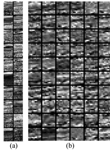
Fig. 9. Filter images learned by an AE on (a) KSC dataset and (b) Pavia dataset. Each N -pixel tiny rectangle stands for N input-to-hidden weights that connects each input unit to a same hidden unit. The intensity of each pixel stands for the absolute value of corresponding weights.
